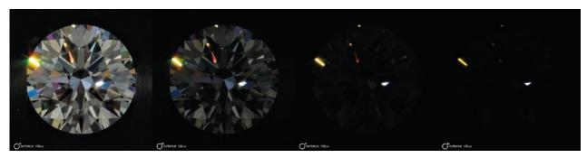
Figure 3.3 A scintillation flash (white) and a fire flash (coloured) with 'bloom' and 'star' effects. Photos were taken in ViBox with different exposure times and only one white LED as a light source.
