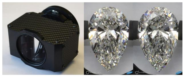
Figure 4.2 On the left is the custom designed stereo splitter that attaches to the end of the macro camera lens. The image on the right side shows a stereo pair of a diamond captured in ViBox with the OctoNus and Lexus watermark logos.
