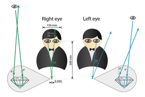
Figure 3.10 Two traces of light rays drawn to suggest light 'coming out' from different eyes and entering the same point on a diamond table. Modern Tolkowsky proportions are used for ray tracing (see Fig. 2.1).
