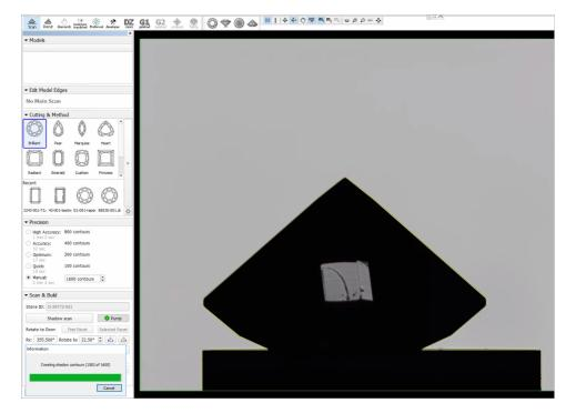
b. After the shadow scan is completed, the model is built based on the scanned contours.
