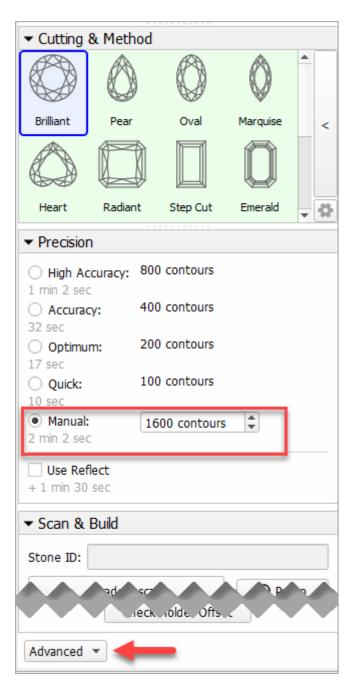
6. To perform shadow and reflect scanning sequentially, check Use Reflect.
