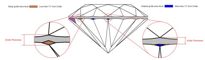
The obtained arrays of values are used to draw the involutes of the girdle surface and to determine the bezel, valley, bezel and bone girdle thicknesses may be measured in at most 16, 8 and 8 points accordingly for most rounded cuts. These girdle thicknesses are measured using a virtual cut without Extra facets.
