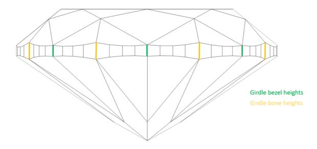
MAX(MAX(Girdle bezel height)-MIN(Girdle bone height), MAX(Girdle bone height)-MIN(Girdle bezel height))
