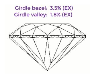
Girdle thickness is measured in 720 directions in steps of 0.5 degrees. The thickness of the girdle and given direction is measured by intersection between the girdle and the vertical plane. The difference between the Z coordinates of these points (along vertical axis) is the final thickness of the girdle in the given direction.
