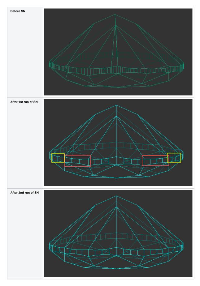
3. The small value of the Shift parameter may block solution search when Custom Facet Marking is enabled.
