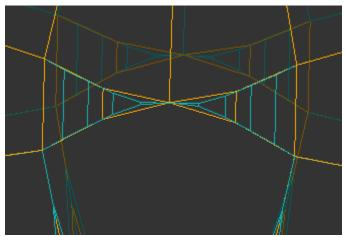
7. Nonconvex heart cuts are supported by Smart Normalize and Smart Recut. However, in the case of Hearts, the algorithm more often has difficulties with the girdle shape and finding the correct symmetry axes for the scanned models. Thus for building Heart allocation forms it is better to use the models created in the Cut Designer or the solutions of Recut or Smart Recut algorithms.
