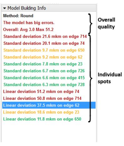
Linear deviation is the maximum deviation of an edge from the corresponding contour.
