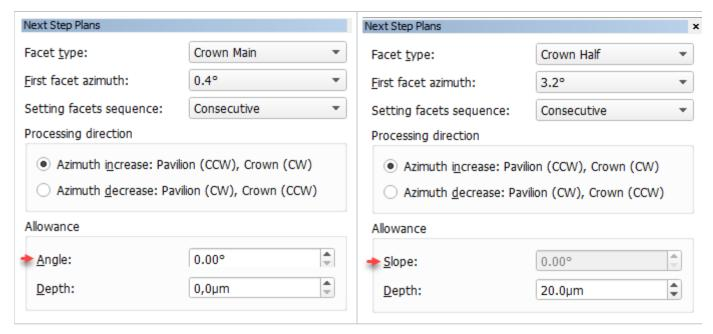
The Slope and Depth default values are now taken from the configuration file (saved there on user input in the corresponding fields).
