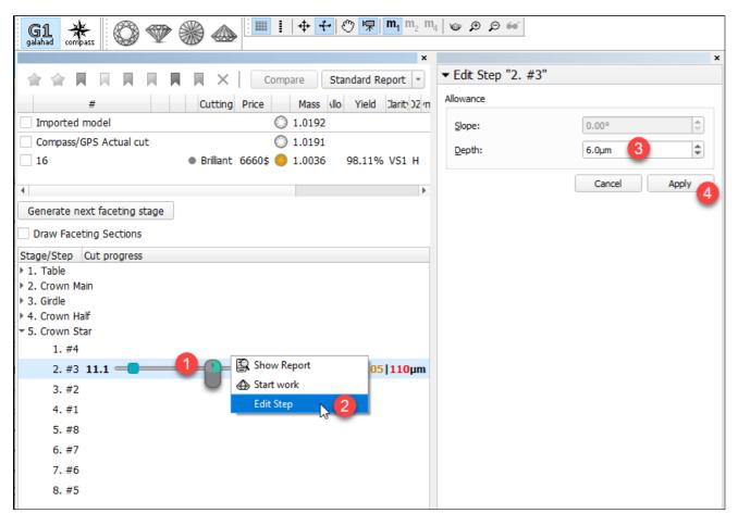
You can do the same for the stage. Note that if some steps of the stage have their own changed allowance, applying a new value for the stage will reset all steps, the corresponding warning is displayed:
