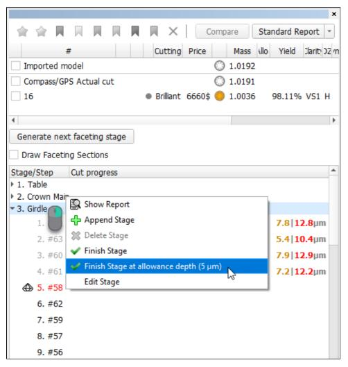
The actual cut of all (remaining) steps is set to the left border of the allowance area. The stage is finished.
