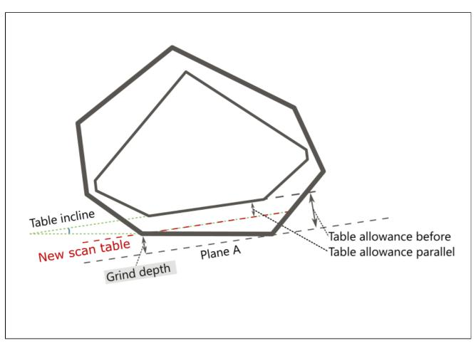
By finding the distance between *Plane A* and *New scan table*, where:
