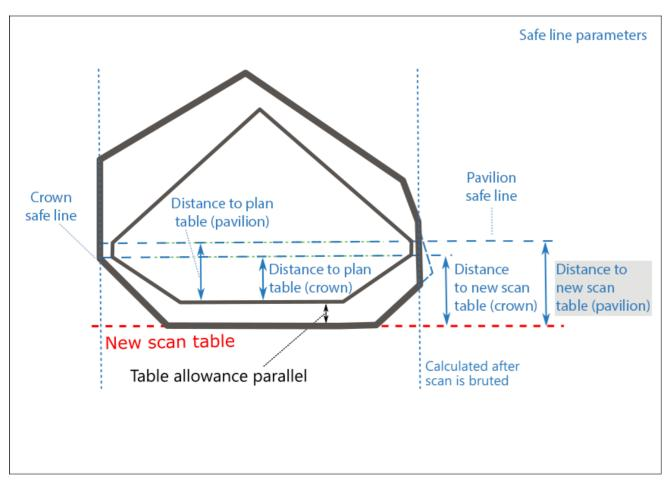
Calculated after the scan is bruted by finding the distance between New scan table and Pavilion safe plane ("line"), where:
