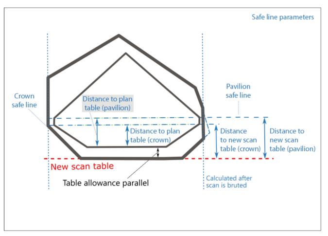
Calculated after the scan is bruted by finding the distance between Pavilion safe plane ("line") and solution table, where:
