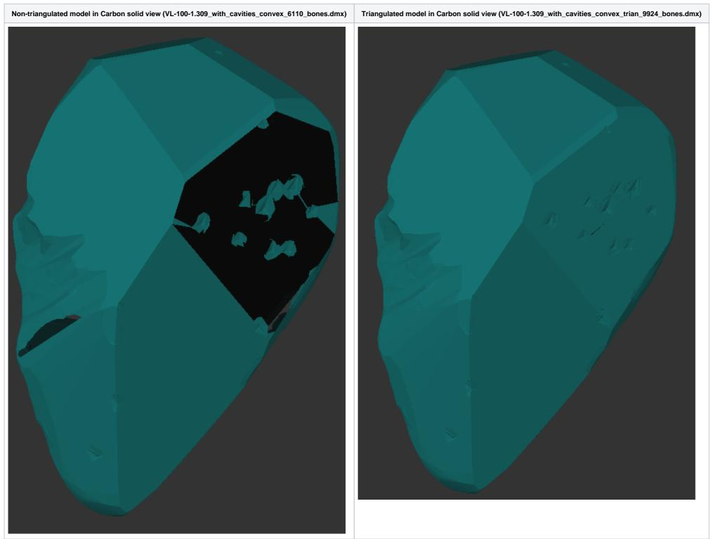
We simplified the topology of resulting model: the cavity area became smoother (with less number of triangles) and intermediate zone between cavity area and convex part became smoother too. Also more shallow cavities are detected automatically in new version. Here you can see the comparison in same model (alpha 46 and 1.0.1.47):
