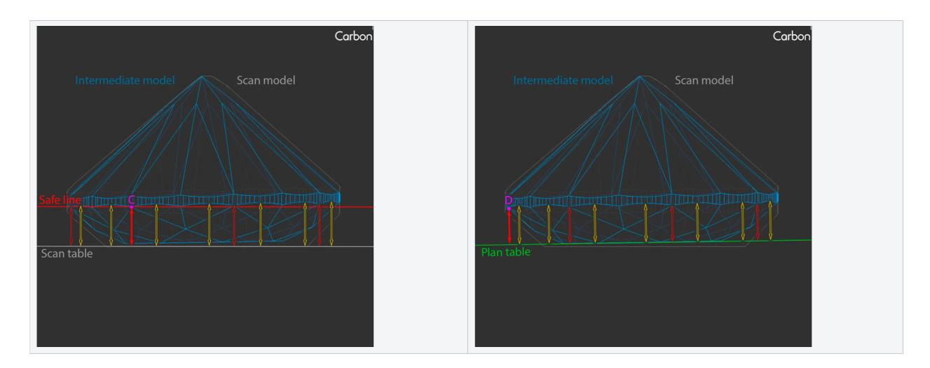
Safe line: Distance to scan table is distance between point C and scan's table plane.
