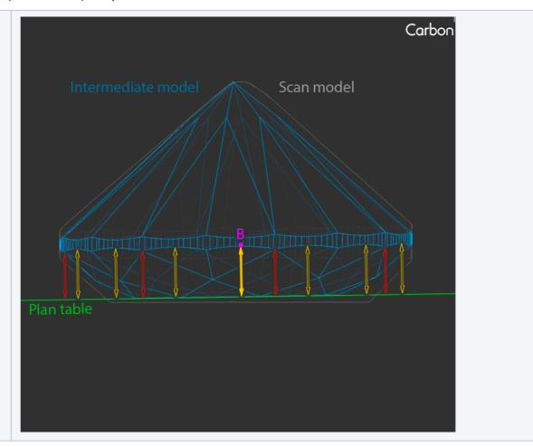
Reference line: Distance to plan table is distance between point B and plan's table plane.
