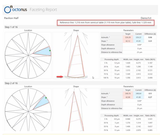
Note that if the "Girdle" or "Table" stages are included in the process, the distance to the reference line is **recalculated** for all other stages.
