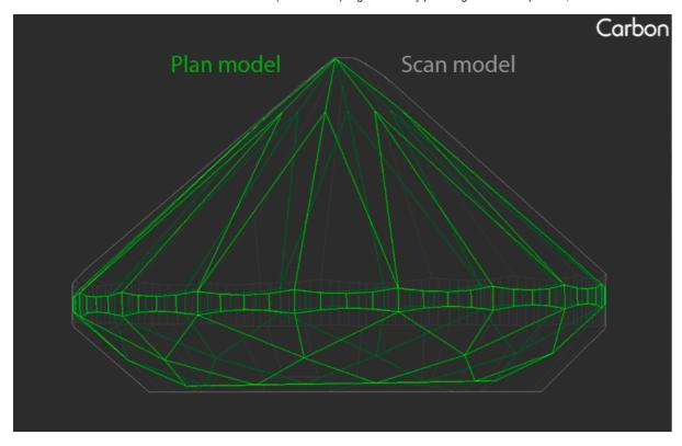
Safe line on Crown is the line of section of the scan's model by the plane passing through point C and parallel to the scan's plane. For each facet on the crown's mains and halves of the intermediate model a point on the facet is determined which is most distant from the scan's plane. From these points the closest to the scan's plane is point C.
