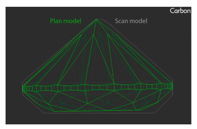
Reference line on Crown is the line of section of the scan's model by the plane passing through point A and parallel to the scan's table. Point A is the point on the crown's mains and halves of the intermediate model, which is most distant from the scan's table plane.
