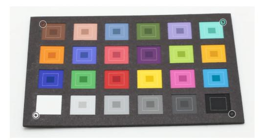
In case of successful profile generation, recognized grid and fiducials (small colored circles at the corners) are displayed on the image thumbnail. Manually adjust fiducials position and click the "Create profile" button in case you are not satisfied with the result of automatic pattern recognition.
