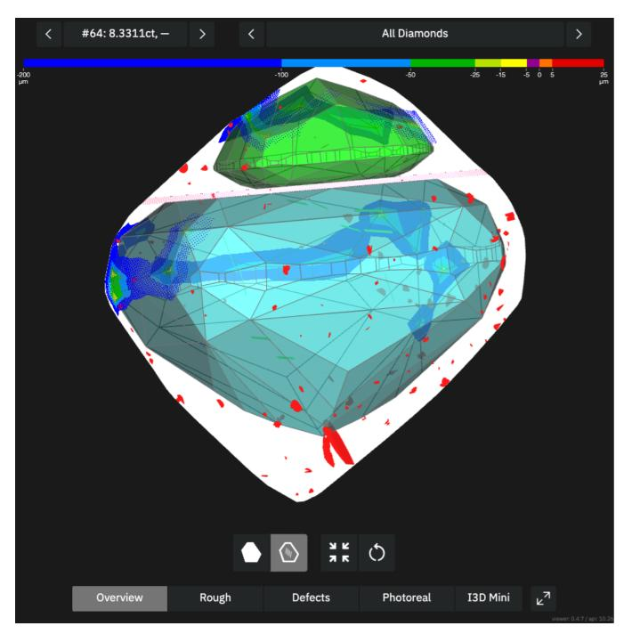
1. All inclusions in rough are shown 2. Colored distance from diamond surface to rough is color coded. This distance marking becomes transparent when viewing angle is close to perpendicular to solution' diamond surface
