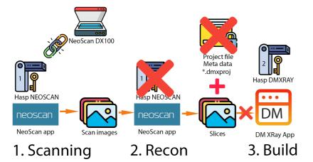
■ The keys also store information about the binding to a specific Neoscan scanner, so the Neoscan HASP must be inserted into the computer to which this specific scanner is connected.
