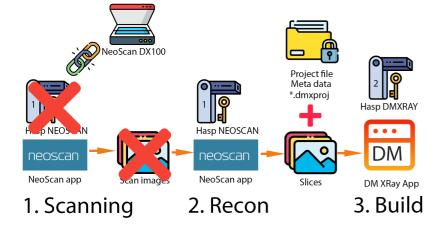
■ The new Neoscan program generates encrypted data during scanning and reconstruction only if HASP Neoscan is inserted; otherwise, the data is saved in an open format, but it cannot be opened in the new DM-XRay Neoscan software.
