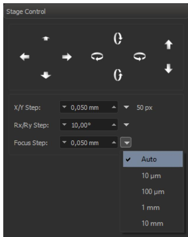
The stage can be moved or rotated by pressing the buttons. Step size (single button press) can be entered into the edit boxes below or can be selected from the corresponding dropdown list.
