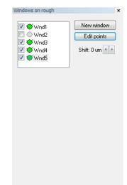
In addition to old windows labeling method that uses 3+ points on the rough surface we have implemented single-point windows labeling. You can see how it works in the complementary video with AutoAdviser demonstration. For both 3+/1 point methods press **New window** button on **Windows on rough** panel, then label window on rough surface and press **Stop edit.** The resulting window is highlighted on the model with light blue color as can be seen on the screenshot below.
