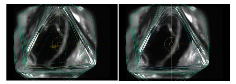
After you have hand labeled windows on rough you can use **Locate Inclusion** panel. Whenever you click on a recommended view direction system automatically changes rough stone position and orientation. See <u>complementary video</u> for detailed demonstration.
