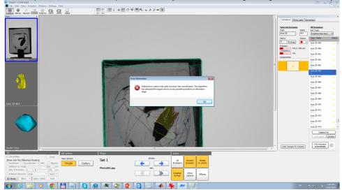
• Inclusion reprojection is not fully on the current image. This case is rare for HIG data, but for Mbox one it may occur. On this image you can see the inclusion that is intersected by the image border, for such inclusions, unfortunately you cannot apply this tool:
