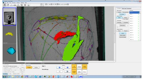
As you can see, using this operation, you may emulate 'Add contour' and 'Subtract contour' options in voxel QC mode. Note that the final accuracy of contour will be lower than for 'Subtract contour', because it is limited to voxel size. That is why in demo voxel QC mode the final accuracy will be lower than in full-resolution voxel QC mode. Anyway we hope that this operation will be very useful because you do not need to switch to polygonal mode to cut inclusion by contour.
