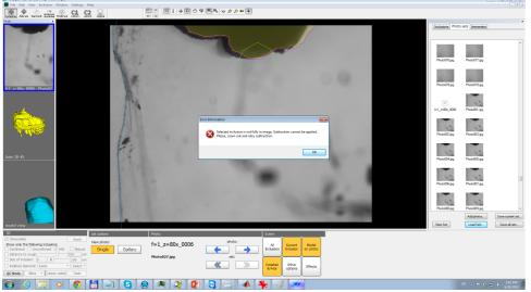
• Hole inside inclusion. Using subtract contour tool you may theoretically make a hole in inclusion (hole is not connected with inclusion surface). Actually we do not recommend to do this. But if for some reason you need to make a hole, please remember that in fact the subtraction algorithm will cut a thin path from hole to the inclusion surface. You can see the result and the thin cut on this image:
