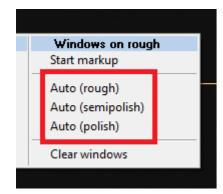
This three menu items are essentially the same windows detection algorithm fine tuned for different types of stones:
