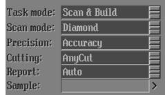
2. For Radiant cutting (POMHR method) Anycut algorithm will be run automatically and program will select better result.
