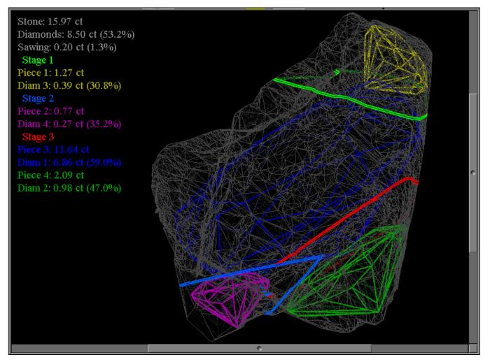
Diamond sawing is divided into a few stages. Each of the stages comprises either a single operation or several operations conducted simultaneously. Only those operations having no particular sequence can be grouped into a single stage. The smaller the reference number of the operation, the earlier it must be conducted.
