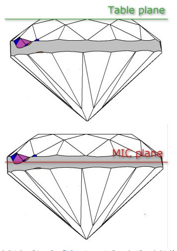
2. In that plane distance from Girdle center mass to diamond out-line calculated for all azimuth.
