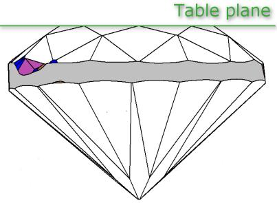
2. Minimum (farest from table plane) and maximum (nearest to table plane) girdle points are detected and search range determined:
