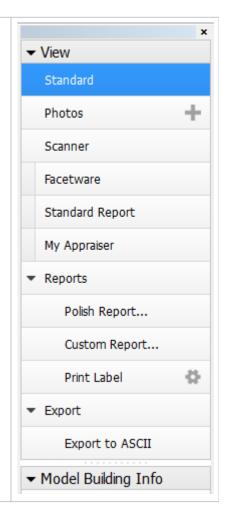
Buttons that control additional panels (Facetware, Standard report, My Appraiser) have an indicator to the left which turns green when the corresponding panel is shown.
