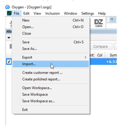
In the Import dialog, select the Recognition option if you want to align the basis of the imported model. This is useful for importing models of the previous gemstone polishing stages
