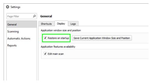
Simply arrange window size and position, go to **Settings General Settings** menu, select **General** section and **Display** tab and click on *Save Current Application Windows Size and Position* button. With *Restore on startup* check-box enabled program will start with remembered size and position:
