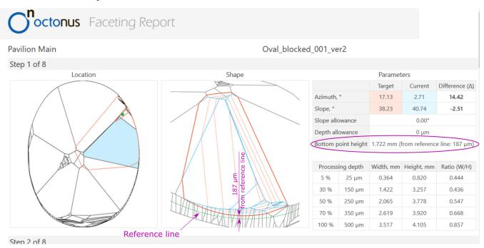
As we can see in the picture above, the bottom point height of the **Step 1** is 1.722 mm and the distance from the reference line to the bottom point is 187 m
