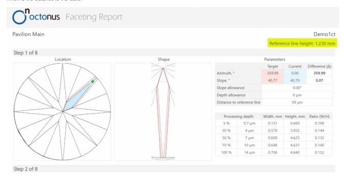
Also, for each facet of the pavilion, the Distance to reference line (µm) is displayed.
