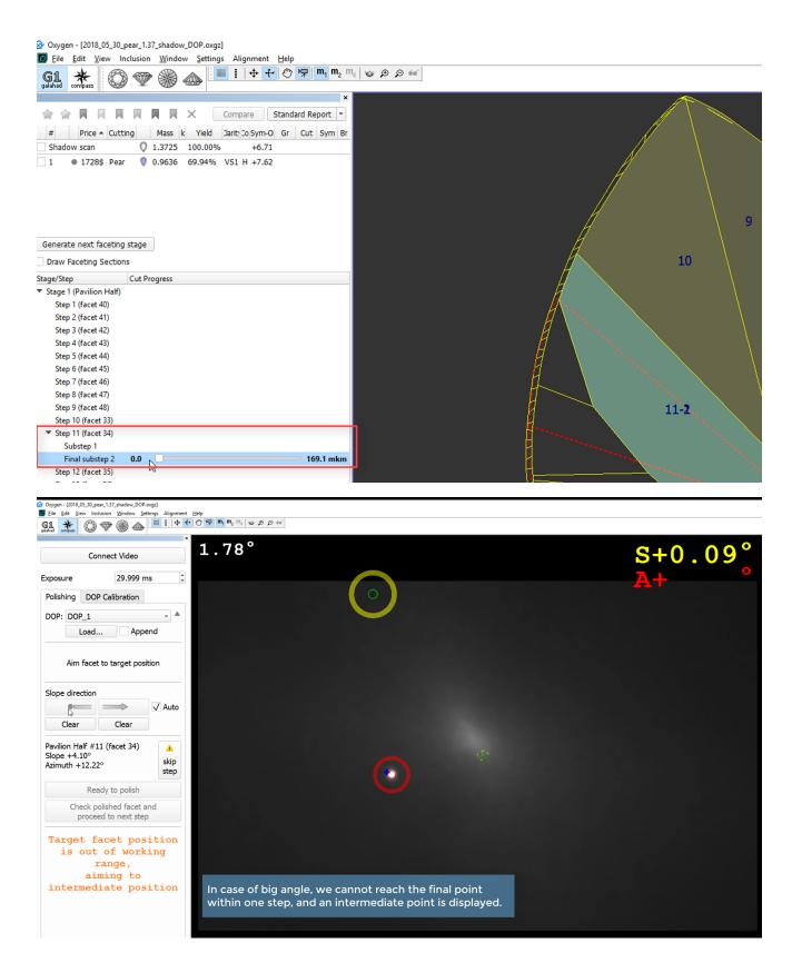
For the big step, two or more sub-steps can be created if necessary. When the polishing is divided between sub-steps, the maximum change is always aimed to be within the initial steps, and the remaining tiny one - in the last step.
