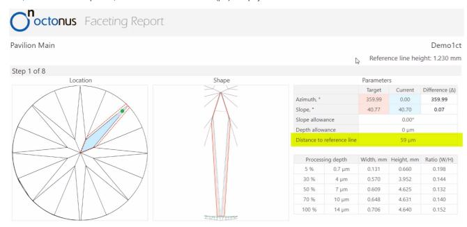
In the same way, the reference line for the crown is calculated. The reference line calculation now considers all the facets of the crown.
