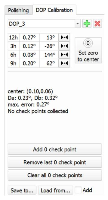
Save results (Save to.. button) and send us obtained the file. Also, send us config.xml.
