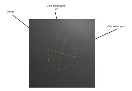
DOP calibration data is built by 4 points, obtained at different angles. When all points collected, there will be a calibration ellipse drawn on the image. It has 4 points marked with crosses, the bigger cross is at "6h" position. Also there will be a dark-green cross, which marks average zero offset (0+). Ellipse parameters are shown in the text box: center coordinates, main diameters values, and the maximum deviation of the current zero offset from ellipse points.
