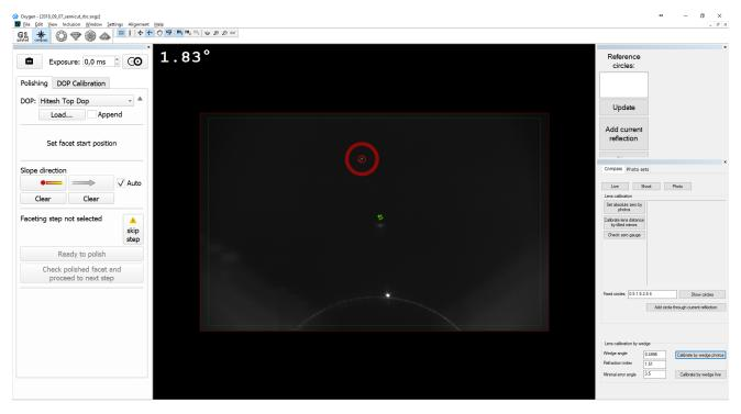
To switch between reflections, you can also use, on the left panel (Compass mode), the Select next reflection button.
