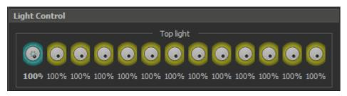
For each type of lighting the panel has its own group of controllers, and the main dial-slider (with star icon).
